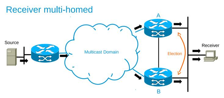
When a Receiver is multi-homed on a LAN, only one of the routers on the LAN should forward the multicast packets on that LAN to avoid duplication
