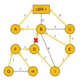
Suppose link between nodes B and D is broken: (for instance, a metal door closes!)
