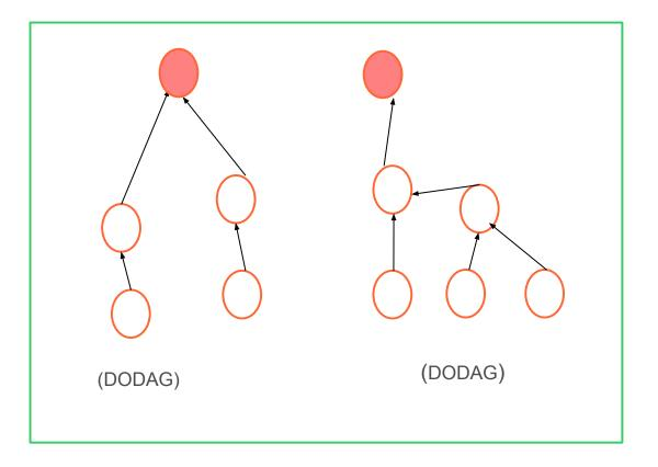
**RPLInstanceID** is a **unique** identifier within a network. DODAGs with the same RPLInstanceID share the same Function (OF) used to compute the position of node in the DODAG.
