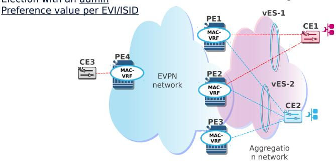
The user must be able to configure a given ES with a "revertive" or "non-revertive" operation. Non-revertive avoids service impact when an ES comes back up.
