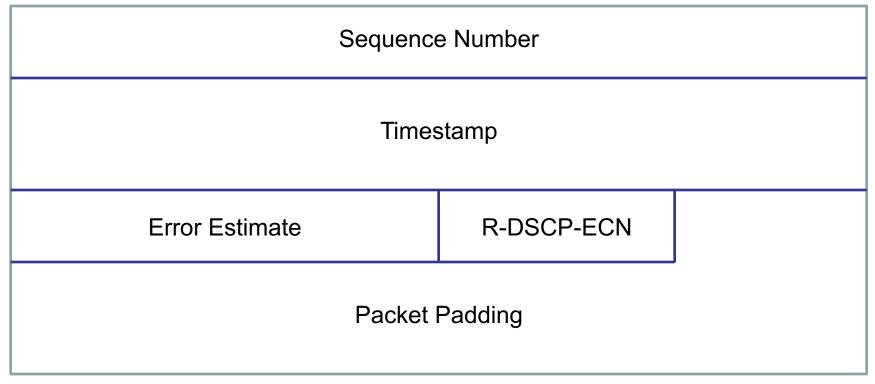
Session-Reflector uses R-DSCP-ECN value to set DSCP field in reflected TWAMP Test packet. DSCP value from the received TWAMP test packet returned in S-DSCP-ECN field of the reflected test packet.
