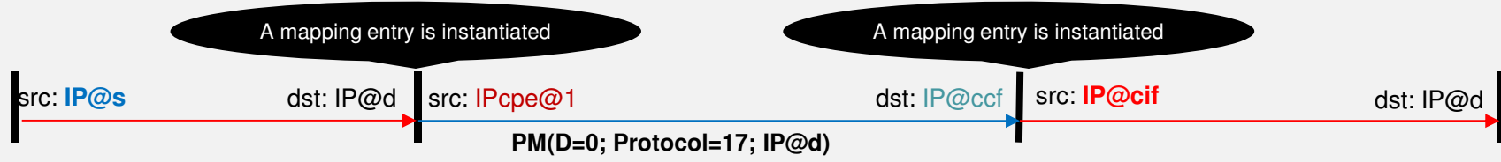
Outgoing UDP packet/without source address preservation at the Concentrator
