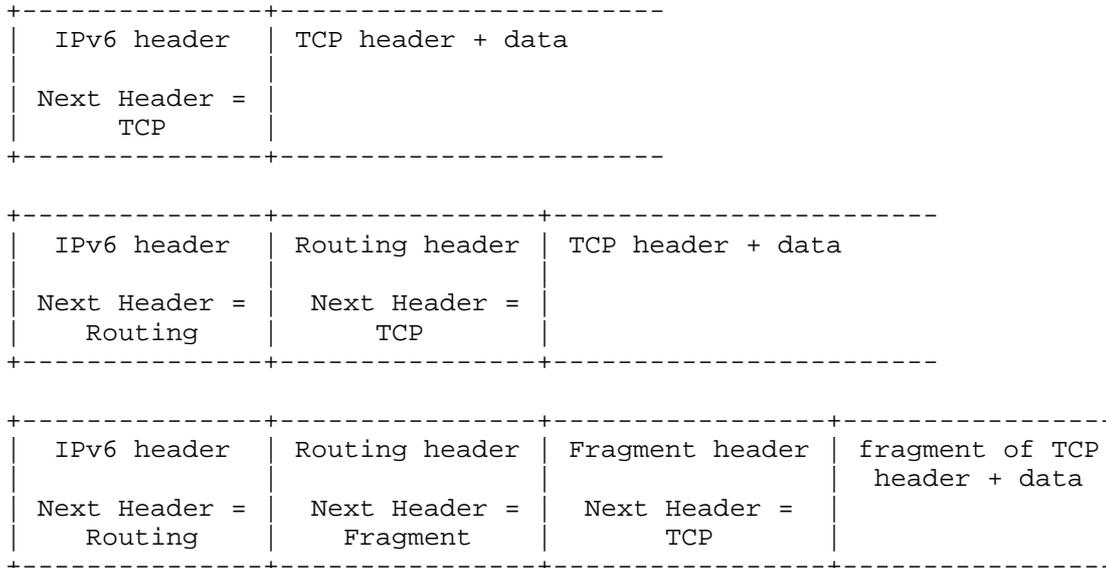
Extension headers (except for the Hop-by-Hop Options header) are not processed, inserted, or deleted by any node along a packet's delivery path, until the packet reaches the node (or each of the set of nodes, in the case of multicast) identified in the Destination Address field of the IPv6 header.
