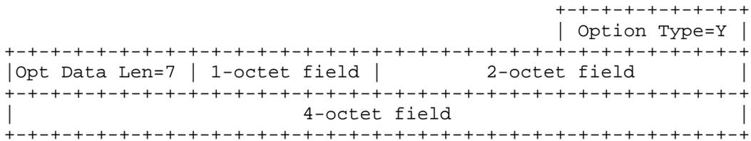
Its alignment requirement is 4n+3, to ensure that the 4-octet field starts at a multiple-of-4 offset from the start of the enclosing header. A complete Hop-by-Hop or Destination Options header containing this one option would look as follows:
