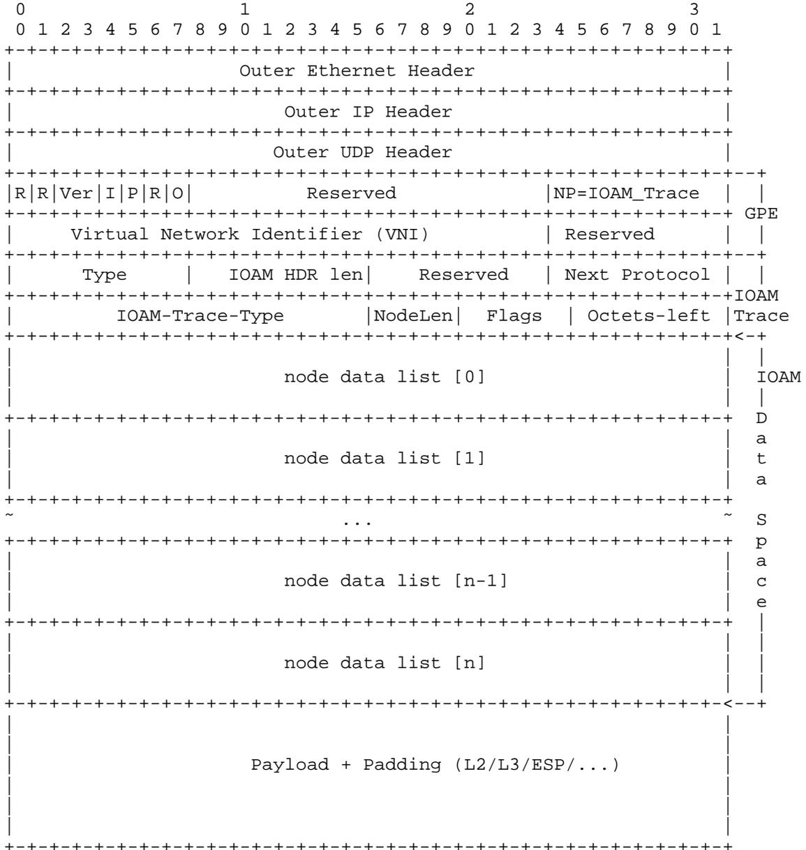
In-situ OAM Trace header following VXLAN GPE header (Incremental IOAM trace):
