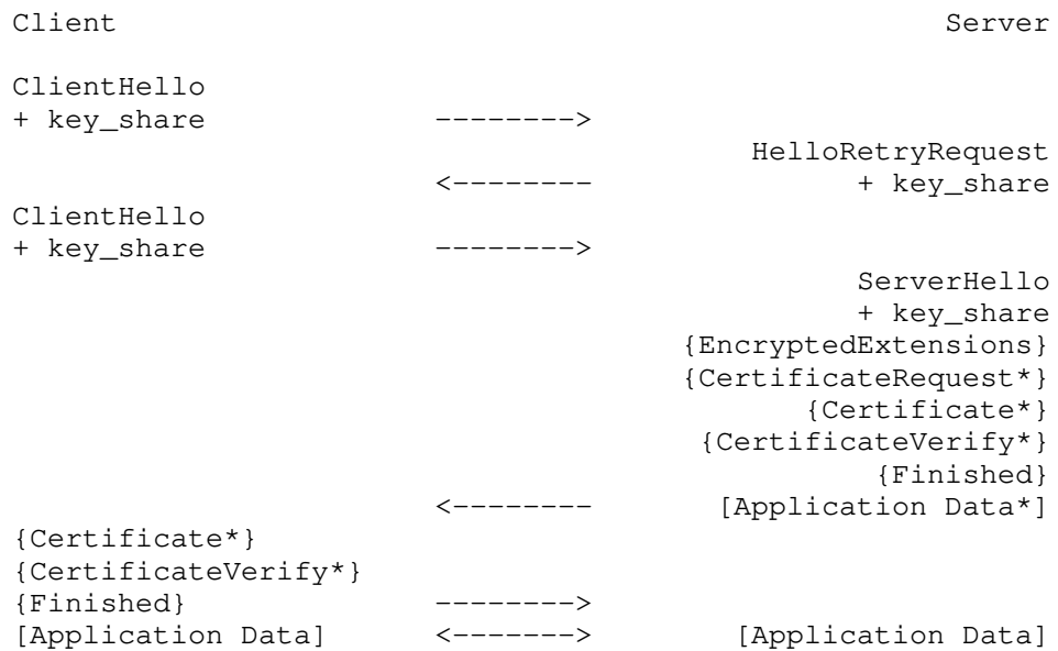
Figure 2: Message flow for a full handshake with mismatched parameters
