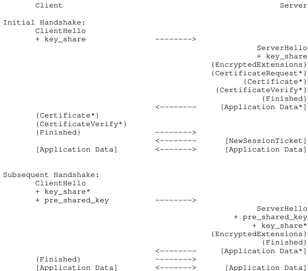
Figure 3: Message flow for resumption and PSK
