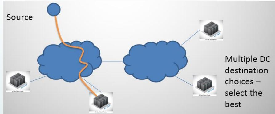
Among a set of endpoints that can meet the customer requirement select the best based on network conditions.
