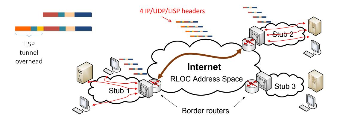
LISP multiplexing and Header compression 1 IP/UDP/LISP header can be shared by *N* packets. Improved efficiency
