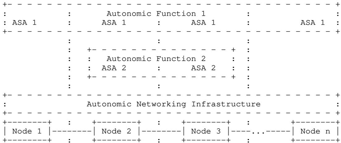
Figure 1: High level view of an Autonomic Network
