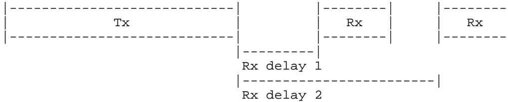
Figure 2: LoRaWAN Class A transmission and reception window
