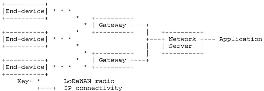
Figure 1: LoRaWAN architecture
