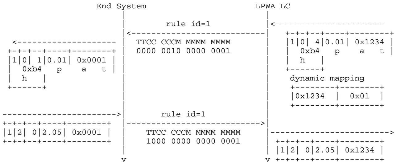
Figure 4: Compression with global addresses
