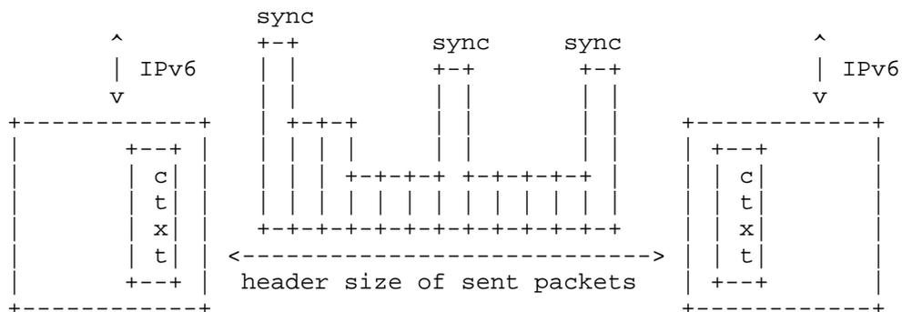
Figure 1: RoHC Compressed Header size evolution.
