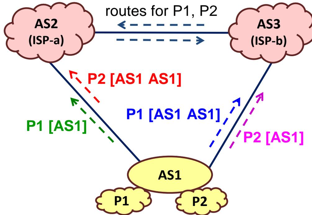
Consider data packet received at AS2 via AS3 that originated from AS1 with source address in P1:
