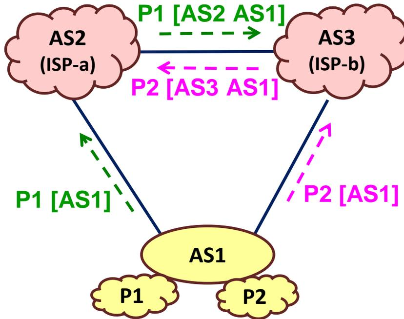
Consider data packet received at AS2 via AS1 or AS3 that originated from AS1 with source address in P1:
