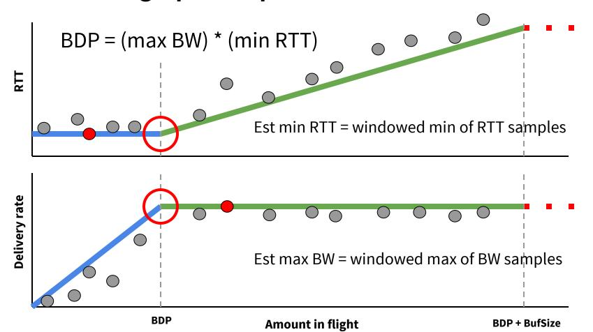
But to see both max BW and min RTT, must probe on both sides of BDP...
