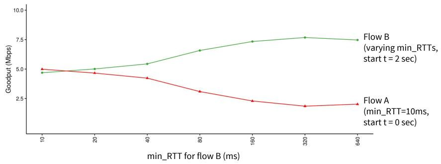
BBR flows w/ higher RTT have an advantage; but BBR flow with 64x higher min\_RTT only has <4x higher bw bw = 10 Mbit/sec, buffer = 1000 packets
