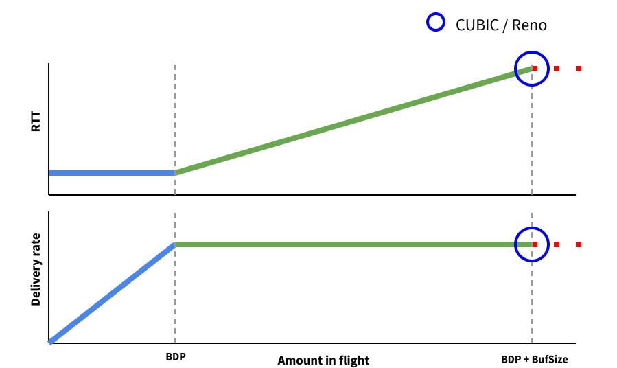
Optimal: max BW and min RTT (Gail & Kleinrock. 1981)
