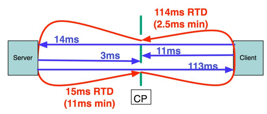
CP to client path has a large delay, could be application or wifi or both. (Same delays affect the server to client delay estimate.)
