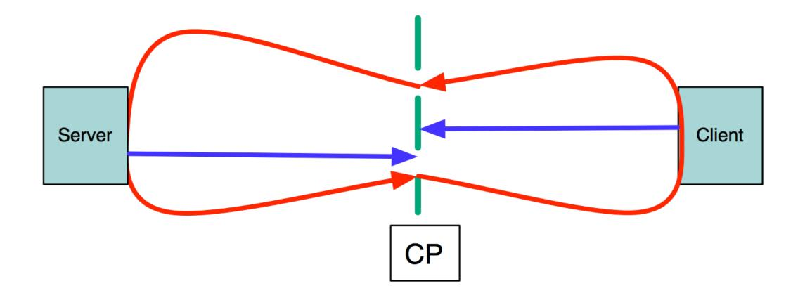
Delay is relative to the packet capture point (CP).
