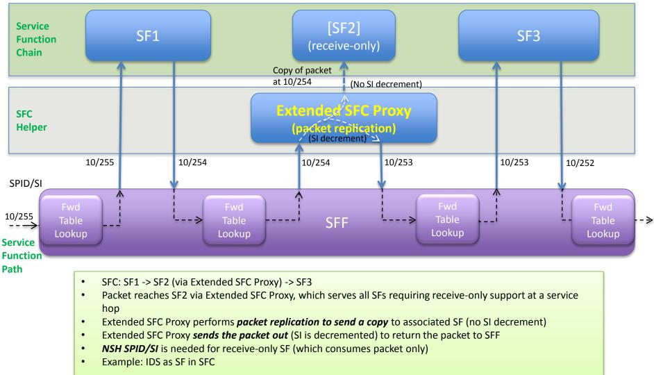
**Extended SFC Proxy functions**: Packet replication, packet forwarding to associated SF (no SI decrement), discard packets from associated SF, packet forwarding to next SF (w/SI decrement).
