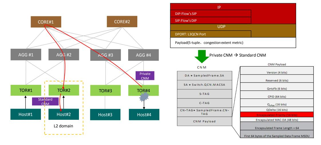
T4 detected the congestion on the port of T4->H4, judge the congested stream. Constructed the private CNM (5-tuple、 congestion extent metric). Encapsulate in IP+UDP. Use the specific UDP port. Set the Dec IP as the Src IP of the stream to make sure the CNM could be routed to the origin TOR.
