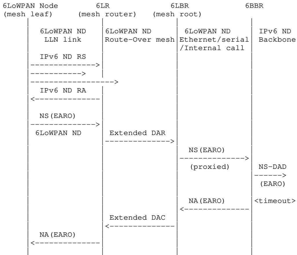
Figure 3: Initial Registration Flow over Route-Over Mesh
