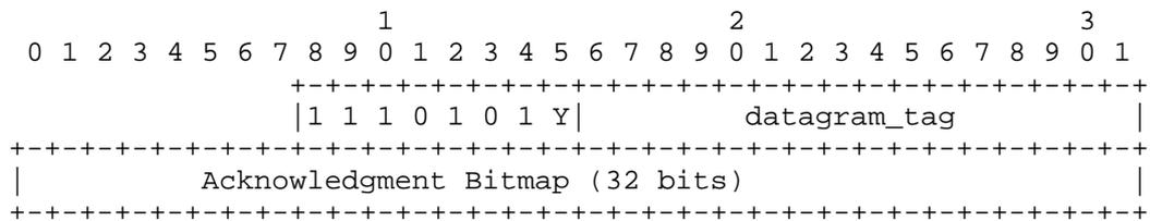
Figure 5: Fragment Acknowledgment Dispatch type and Header
