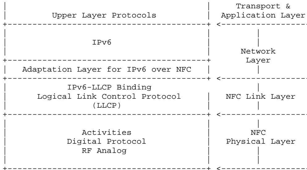
Figure 2: Protocol Stacks for IPv6 over NFC
