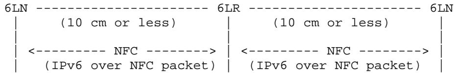
Figure 12: Isolated NFC-enabled device network
