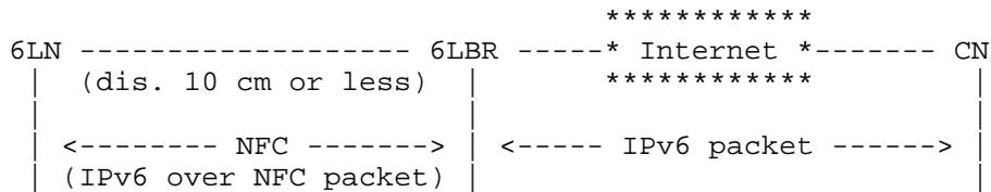
Figure 11: NFC-enabled device network connected to the Internet
