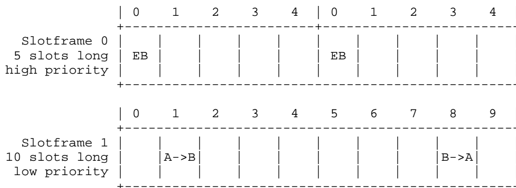
Figure 3: 2-slotframe structure when using 6top alongside the Minimal 6TiSCH Configuration.
