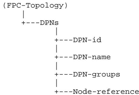
Figure 3: DPNs Model Structure
