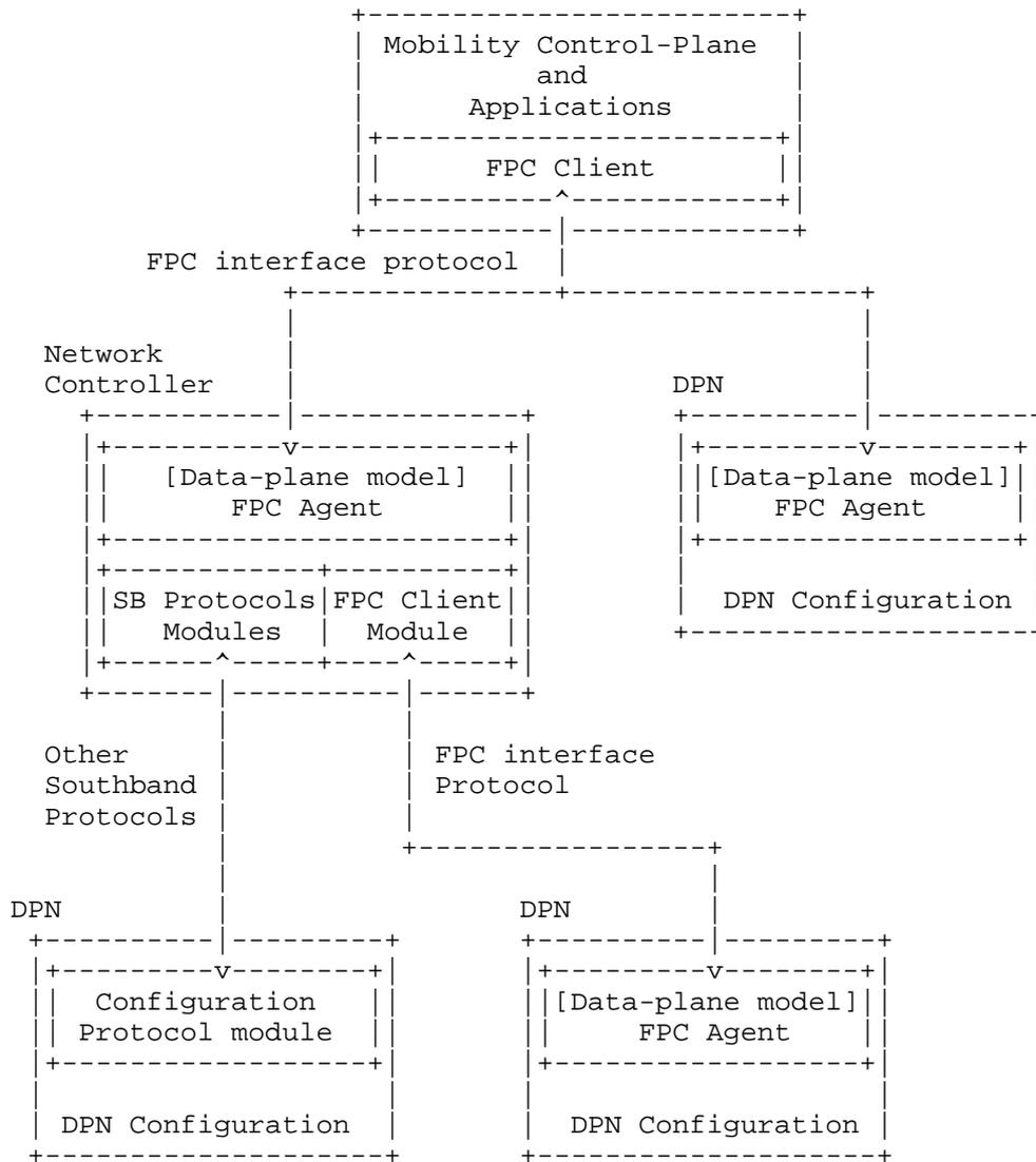
Figure 1: Reference Forwarding Policy Configuration (FPC) Architecture
