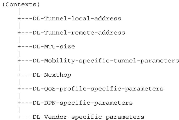
Figure 14: Downlink Context Model of Single DPN Structure
