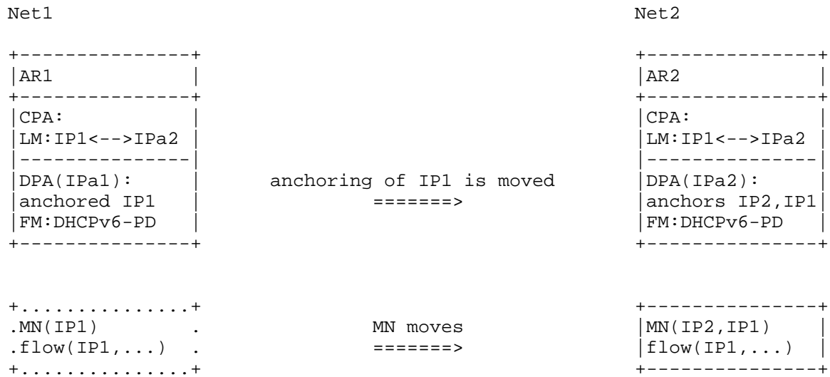
Figure 8. IP prefix/address anchor switching to the new network. MN with flow using IP1 in Net1 continues to run the flow using IP1 as it moves to Net2.
