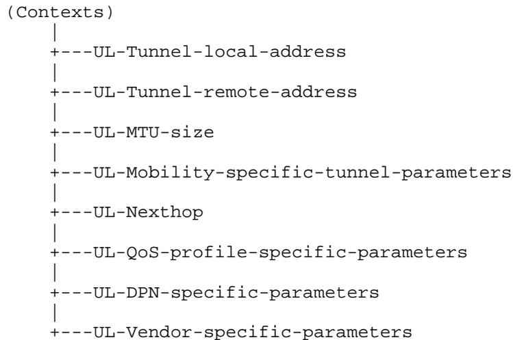
Figure 13: Uplink Context Model of Single DPN Structure
