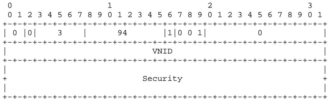
In the above example, the first flag bit is set which indicates that the VNID extension is present this is a 32 bit field. The second through fourth bits of the flags are paired flags that indicate the presence of a security field with eighth possible sizes. In this example 001 indicates a sixty-four bit security field.
