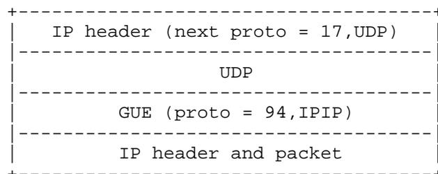
The receiver removes the UDP and GUE headers and sets the next protocol field in the IP packet to IPIP, which is derived from the GUE proto field. The resultant packet would have the format:
