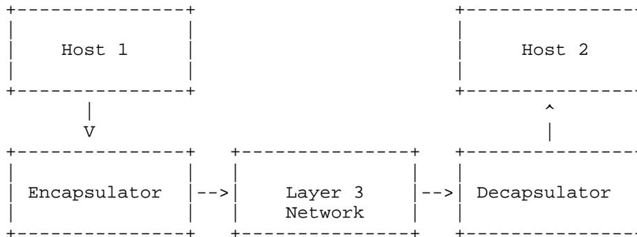
The encapsulator and decapsulator may be co-resident with the corresponding hosts, or may be on separate nodes in the network.
