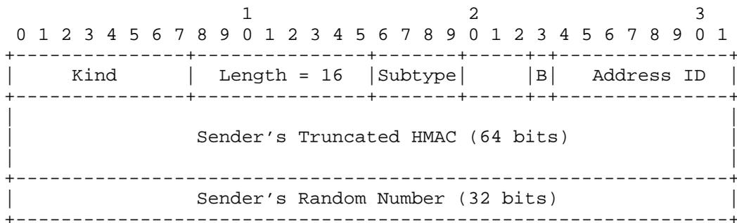
Figure 6: Join Connection (MP\_JOIN) Option (for Responding SYN/ACK)
