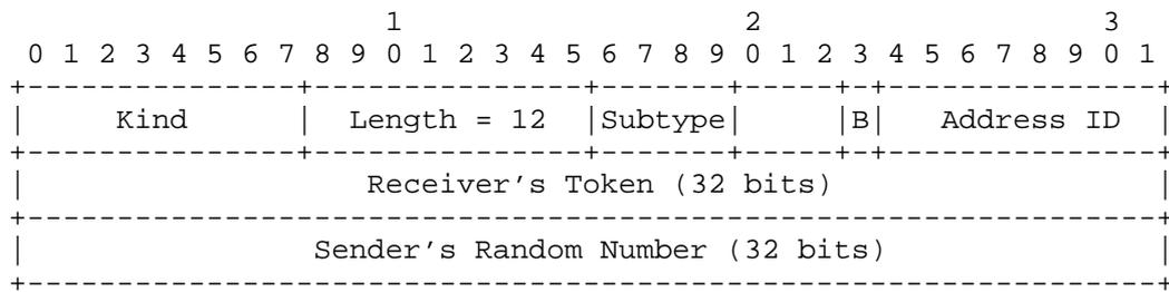
Figure 5: Join Connection (MP\_JOIN) Option (for Initial SYN)
