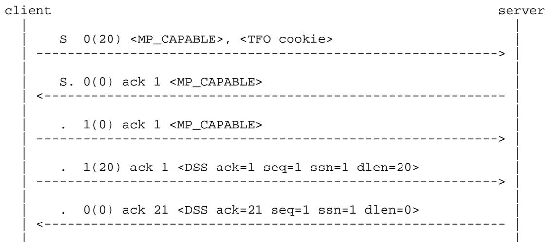
Figure 20: The server does not support TFO
