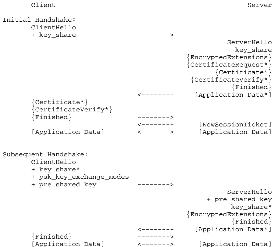
Figure 3: Message flow for resumption and PSK
