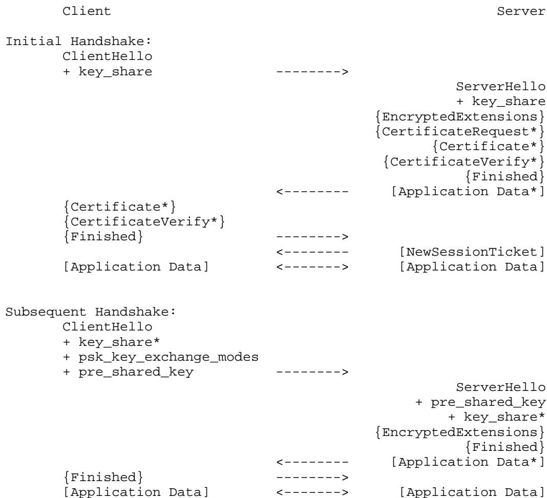
Figure 3: Message flow for resumption and PSK
