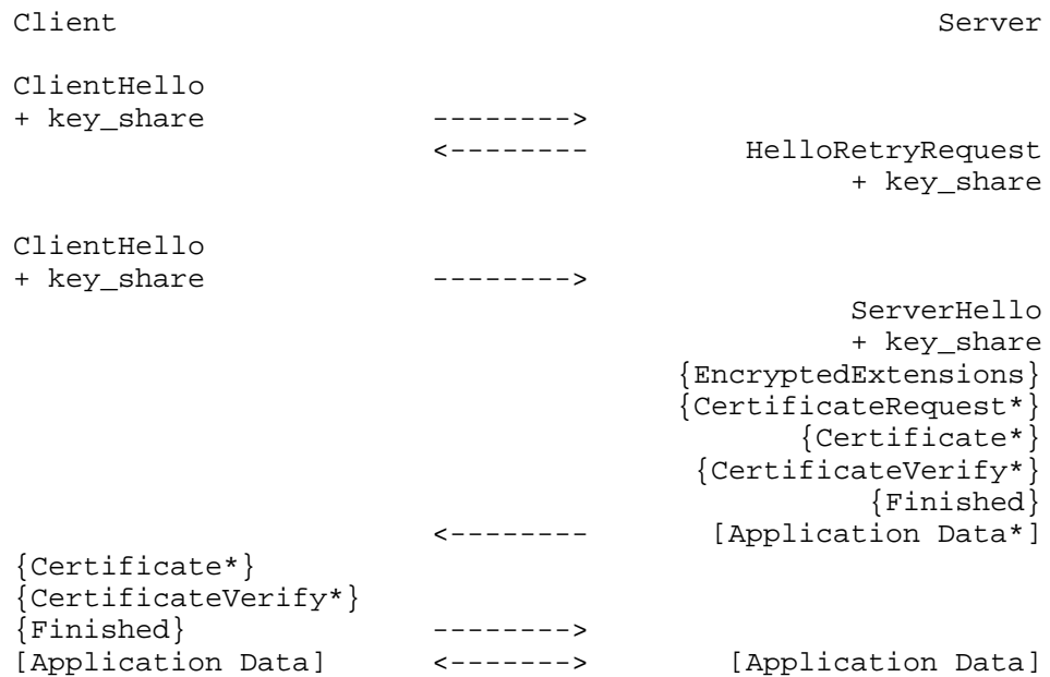
Figure 2: Message flow for a full handshake with mismatched parameters
