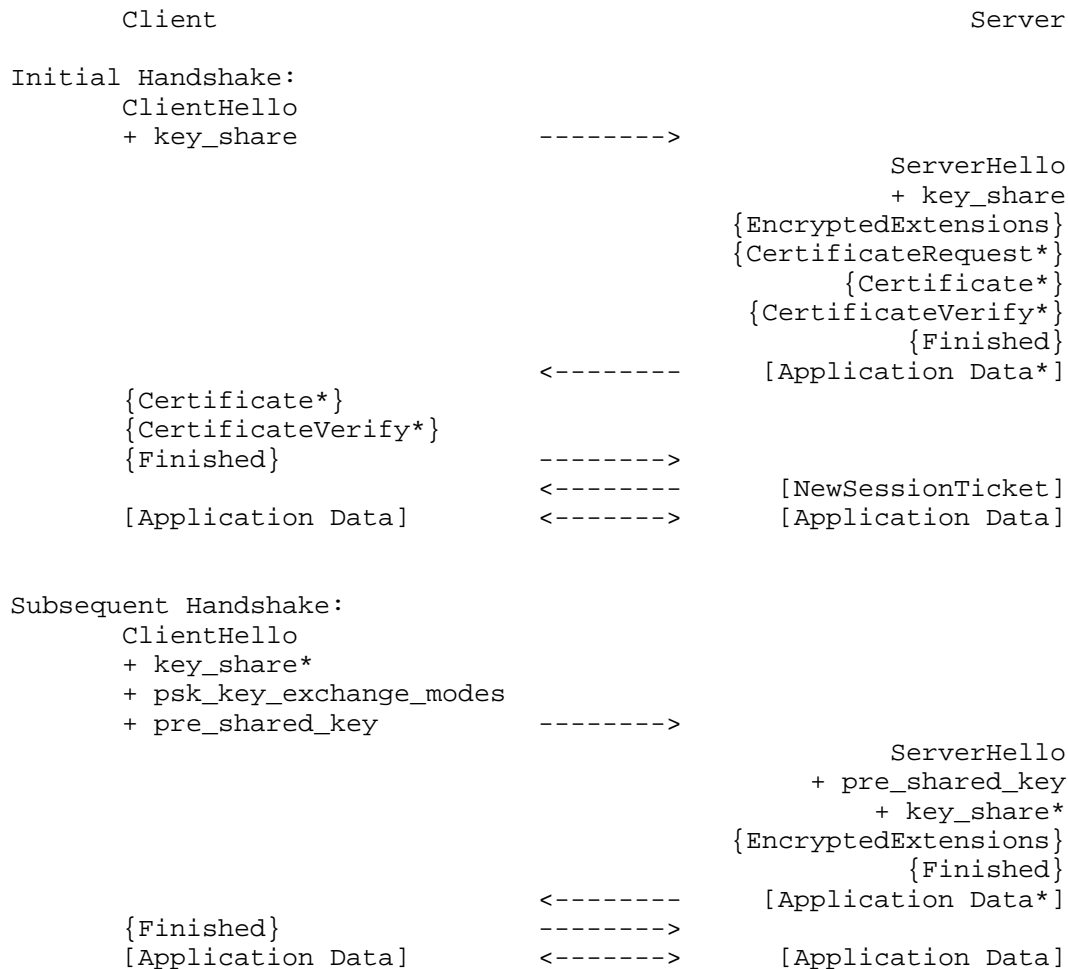
Figure 3: Message flow for resumption and PSK
