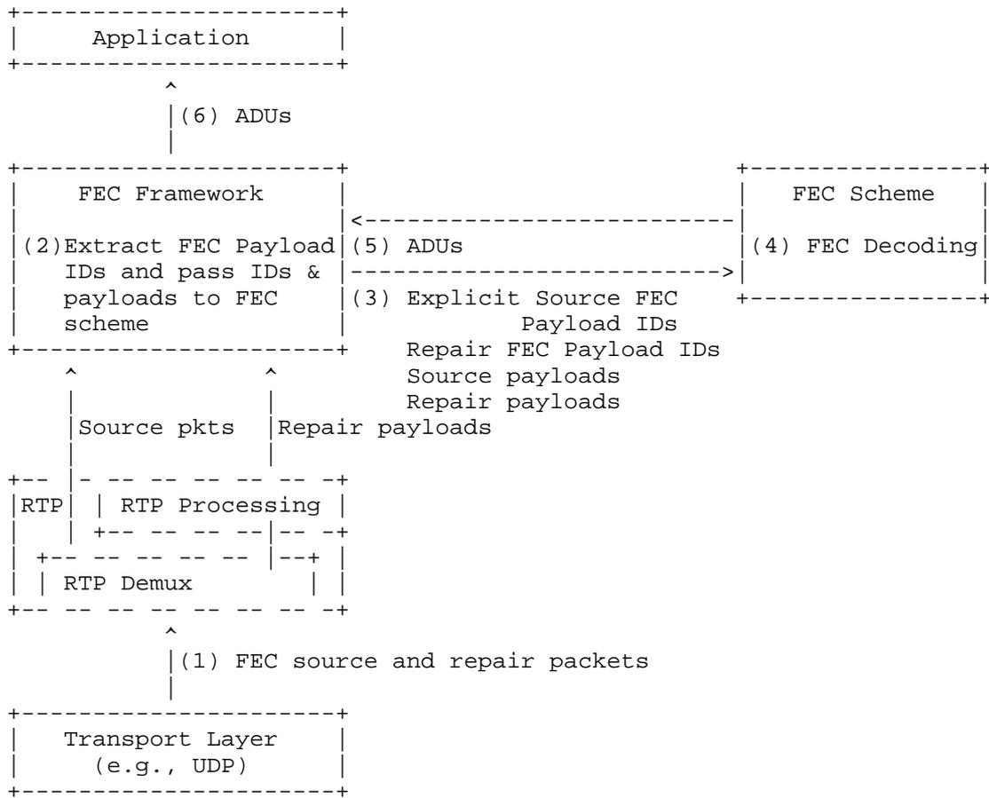
Figure 5: Receiver Operation with RTP Repair Flows
