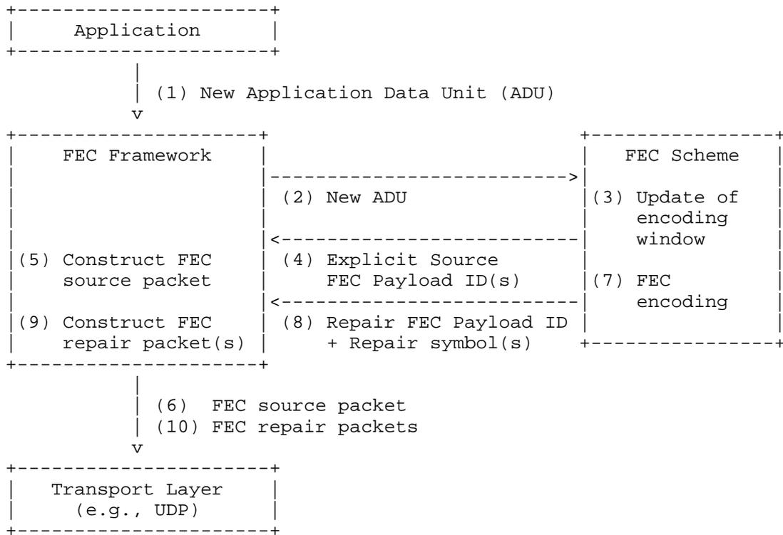
Figure 2: Sender Operation with Convolutional FEC Codes
