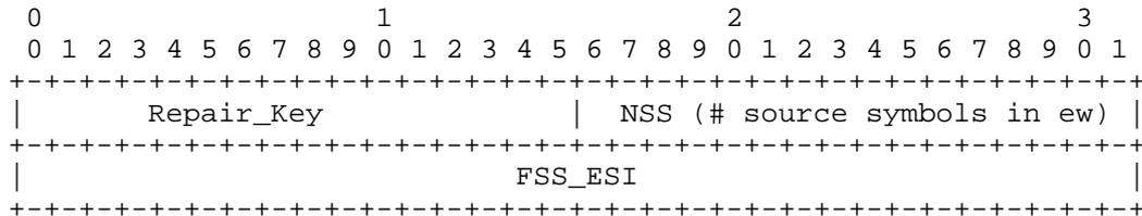
Figure 7: Repair FEC Payload ID Encoding Format
