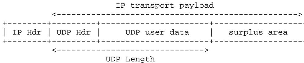
Figure 3 IP transport payload vs. UDP Length
