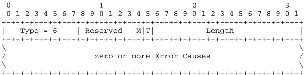
The ABORT chunk is extended to add the new 'M-bit'. The M-bit indicates to the receiver of the ABORT chunk that the chunk was not generated by the peer SCTP endpoint, but instead by a middle box.
