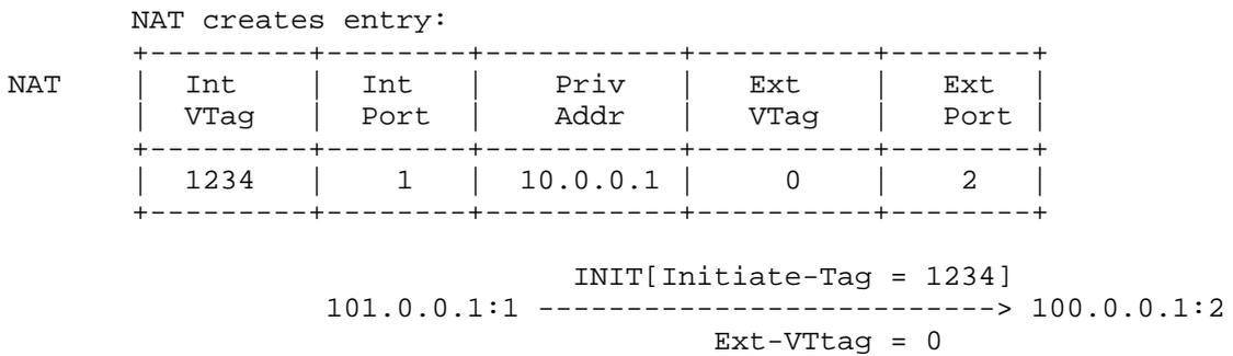
Host B receives the INIT and sends an INIT-ACK with the NAT's external address as destination address.
