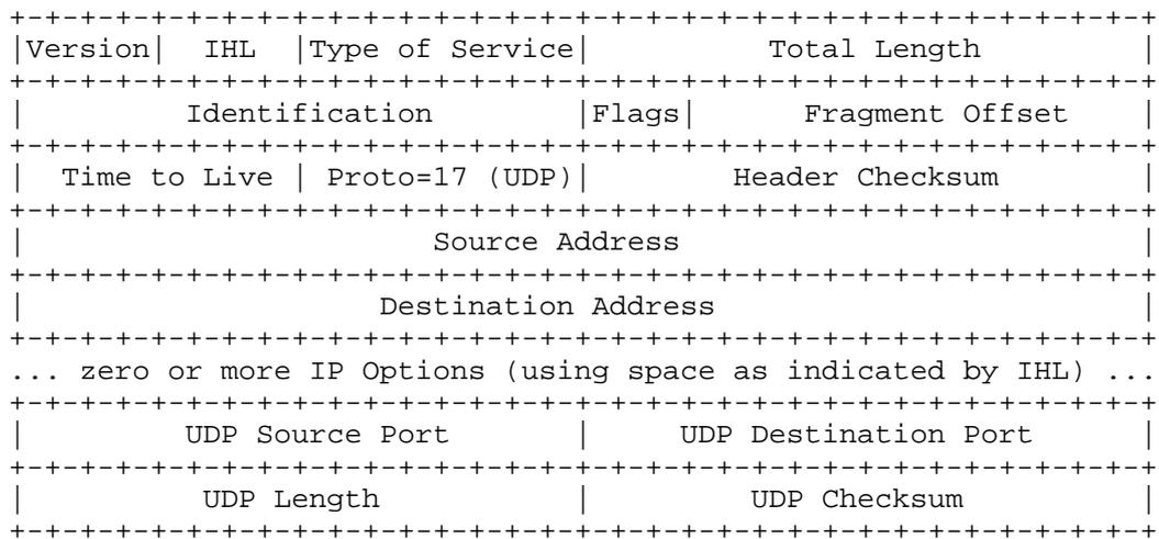
Figure 1 IPv4 datagram with UDP transport payload
