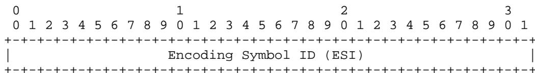
Figure 5: Source FEC Payload ID Encoding Format
