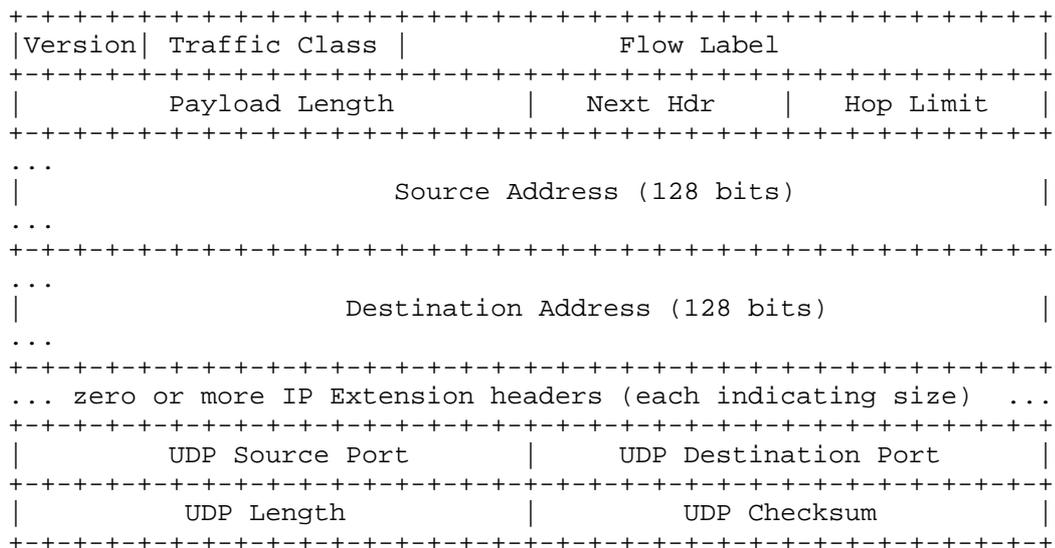
Figure 2 IPv6 datagram with UDP transport payload
