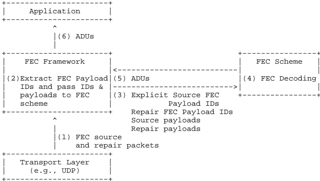
Figure 4: Receiver Operation with Sliding Window FEC Codes
