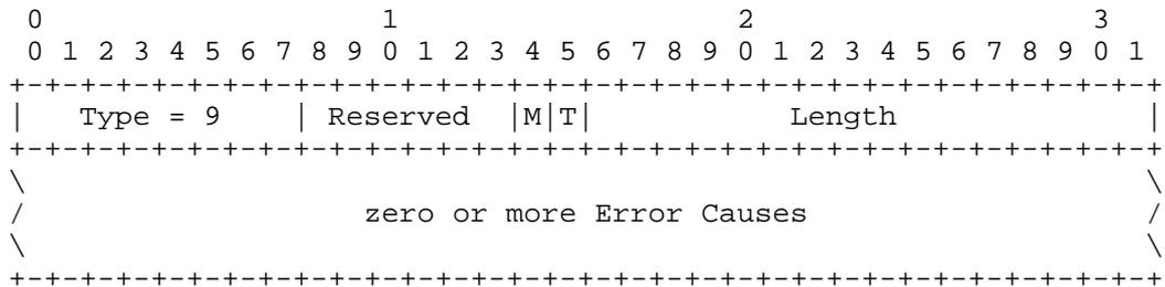
The ERROR chunk defined in [RFC4960] is extended to add the new 'M-bit'. The M-bit indicates to the receiver of the ERROR chunk that the chunk was not generated by the peer SCTP endpoint, but instead by a middle box.
