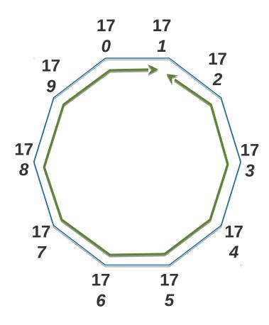
A full ring LSP has the further advantage of simple end-to-end OAM: node 1 periodically sends an LSP ping message to itself. As long as it receives these messages, it's happy – the end-to-end LSP is working.
