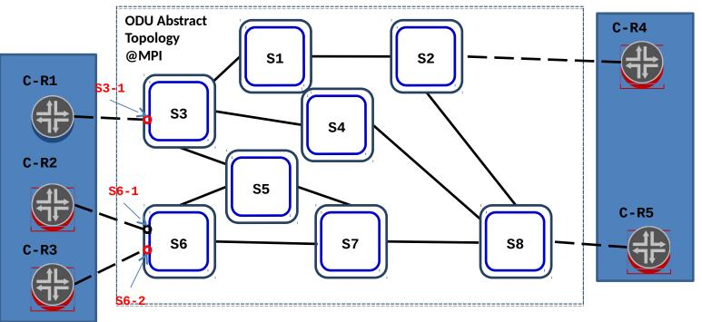
PNC exports as abstract topology at MPI: TE nodes (since the white topology abstraction is used, they represents physical nodes), TE links (between TE nodes), access-links (facing transport border nodes), transport border nodes and link termination points (LTPs) (e.g.S3-1 and S6-2)
