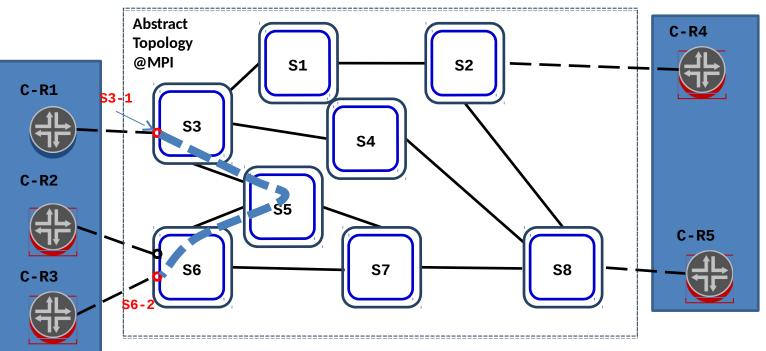
MDSC should request Transport PNC to setup an ODU2 Tunnel (Segment) between S3-1 and S6-2 Ingress and egress points are indicated in the explicit-route-objects of the primary path:
