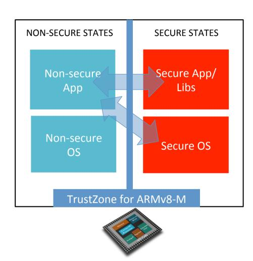
Secure transitions handled by the processor to maintain embedded class latency
