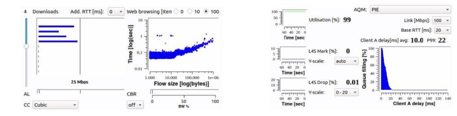
Limited drop and delay for short flows Short flow variations vary around queue target
