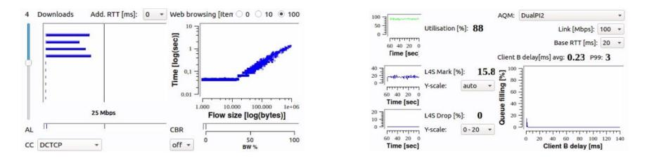
No drop and ultra low delay for short flows Short flow variations are below queue target
