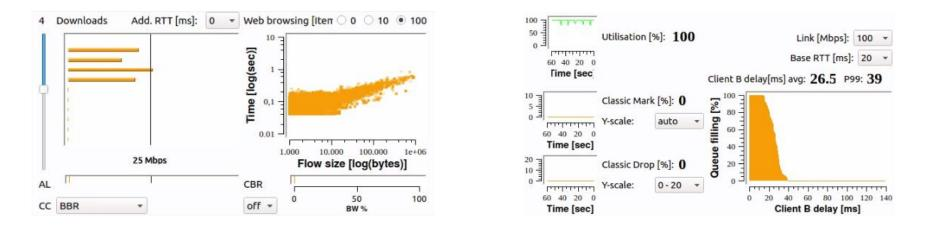
No drop and limited delay for short flows Short flow variations build on top of queue target
