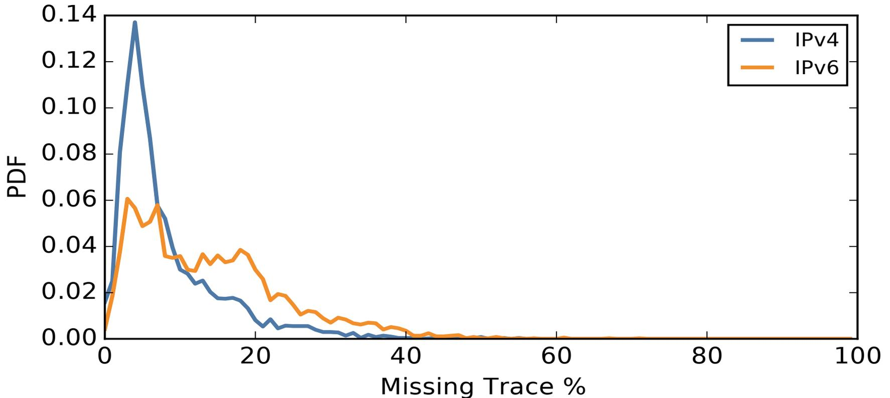
Many more missing hops in IPv6 traces, whether we aggregate over source or over target.
