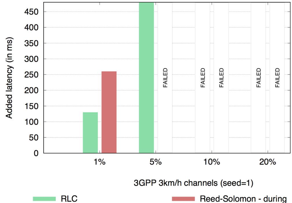
more channels are supported by RLC, and **the added latency to good receivers is far below the maximum 480 ms latency budget**
