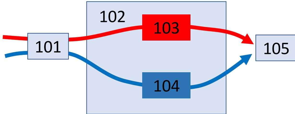
In **VPN A** we allocate path (101, 102, 103, 105), and in **VPN B** we allocate path (101, 102, 104, 105).
