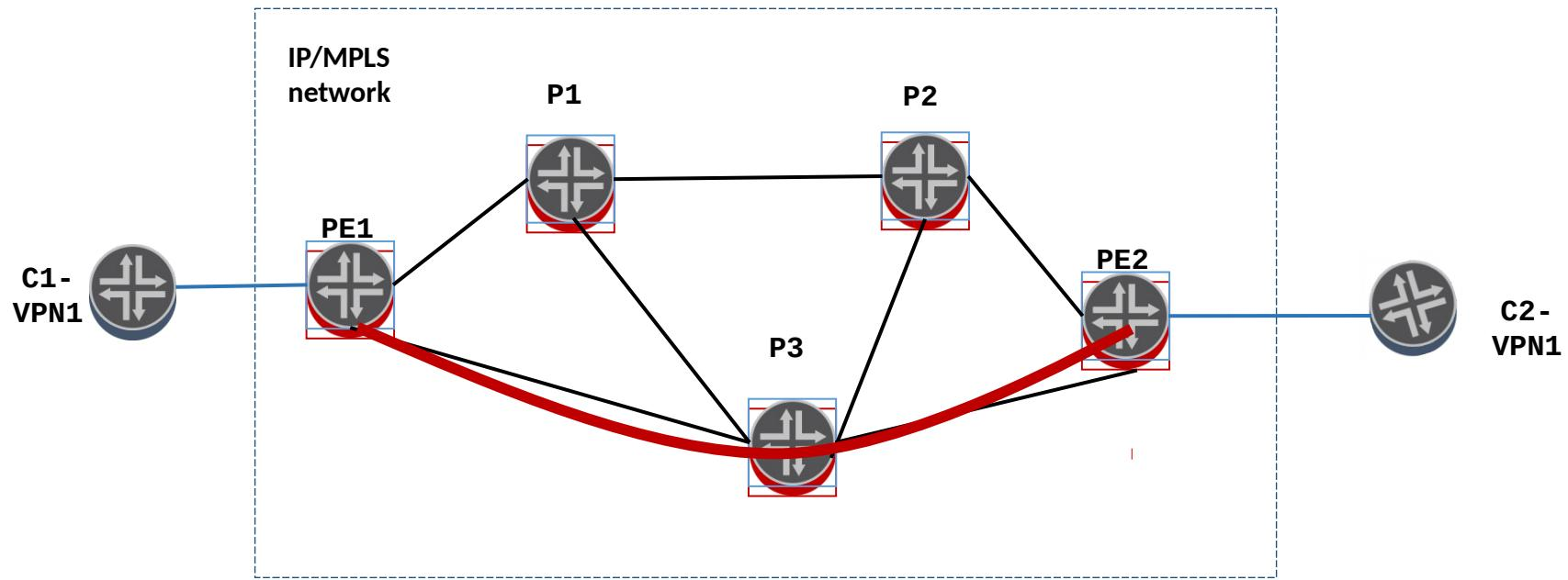
VPN1 VRFs (SFs) on PE1 and PE2 are connected via LSP carried inside delay constrained RSVP-TE tunnel
