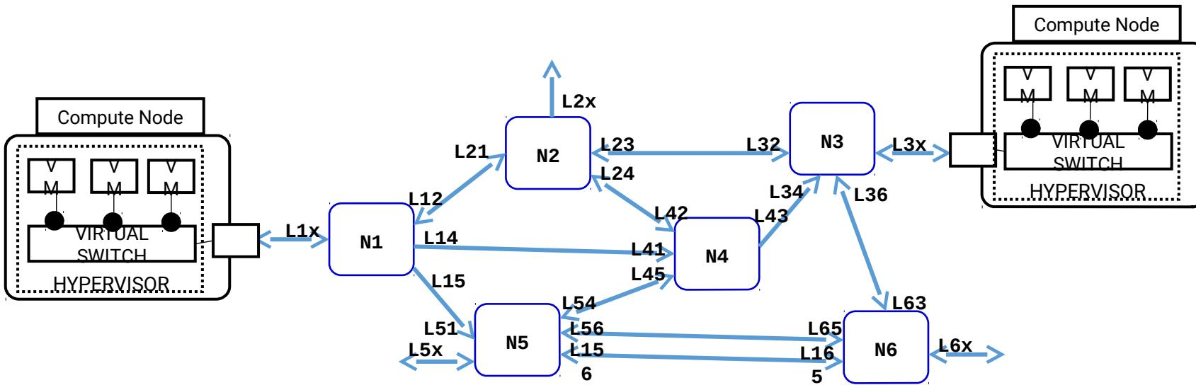
Compute Node is attached to network WAN node. It contains VMs which can be modeled as a Service Function (SF). VM resources (instances, usage, CPU/Memory) can be modeled and integrated with network topology model to facilitate VM migration, dynamic load balancing, etc.
