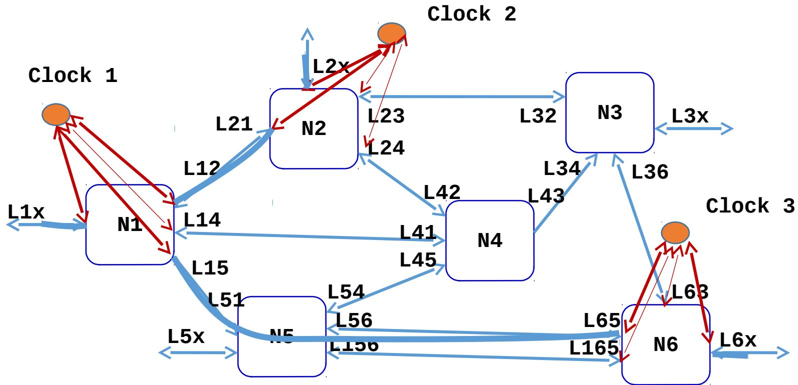
High resolution clock synchronization channels set over TE topology optimized by smallest delay variation criterion
