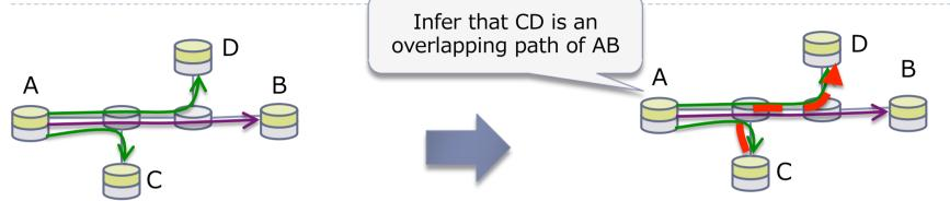
Step 1: Node A checks the routerlevel paths to node B, C, and D.
