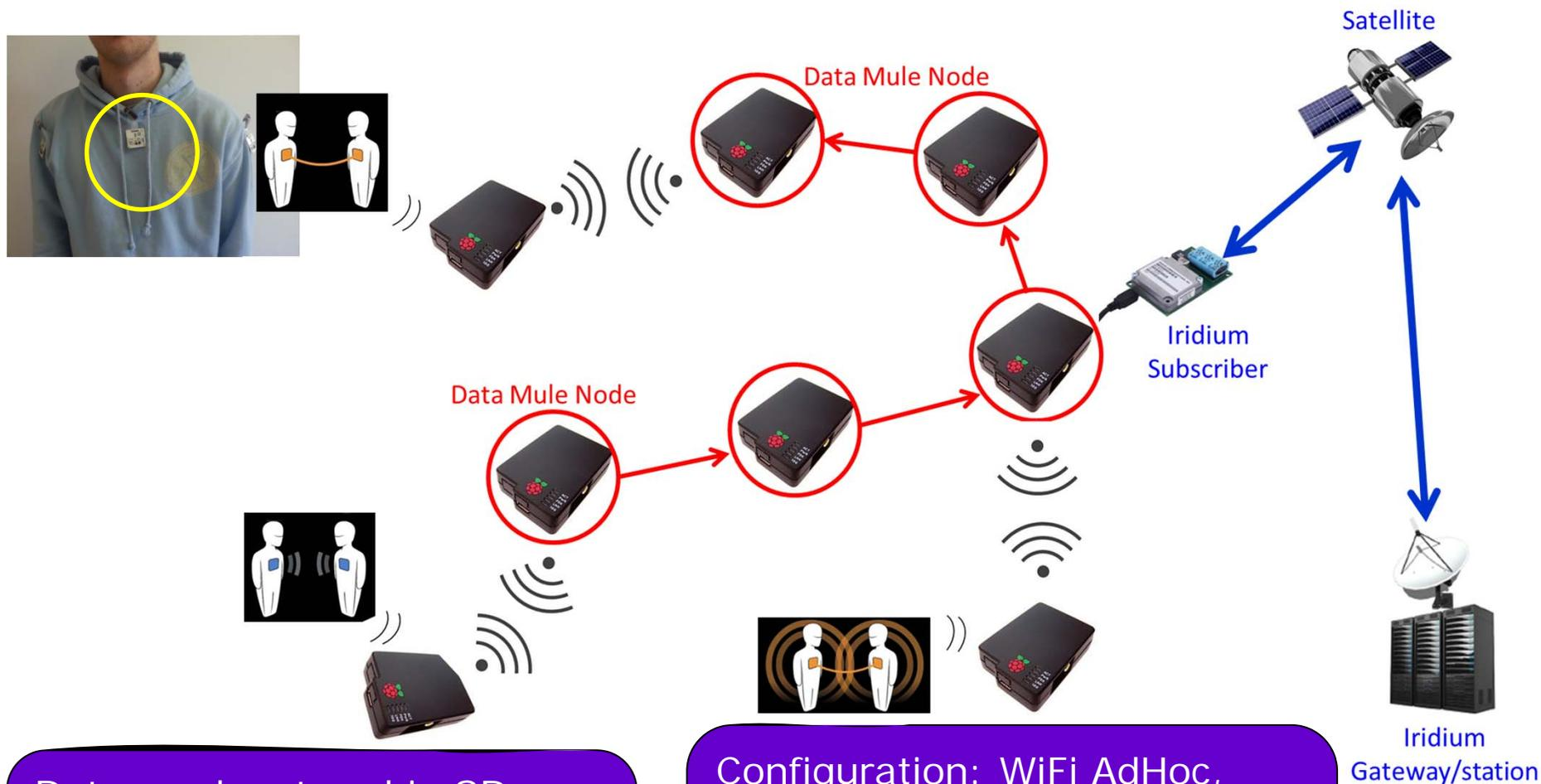
Data can be stored in SD card, transmitted to Data Mule node, or use of WiFi AdHoc mode transmission to Gateway
