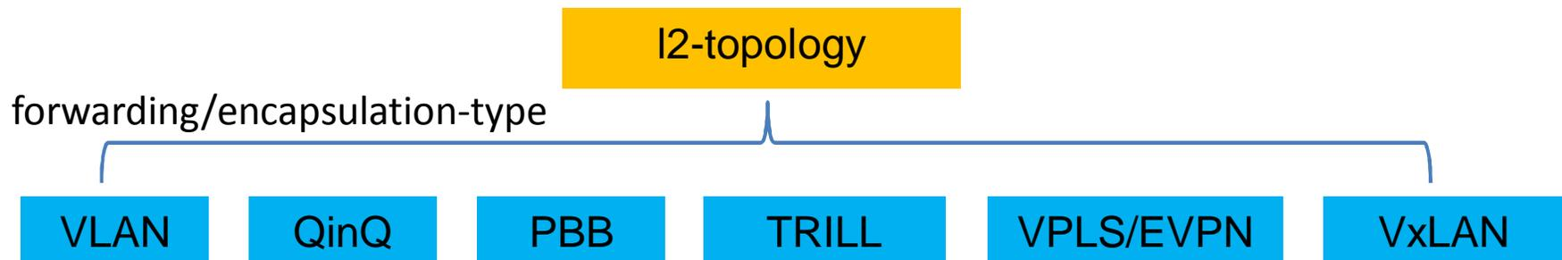
“ Different layer-2 technologies may be enabled on different ports in one L2 topology
