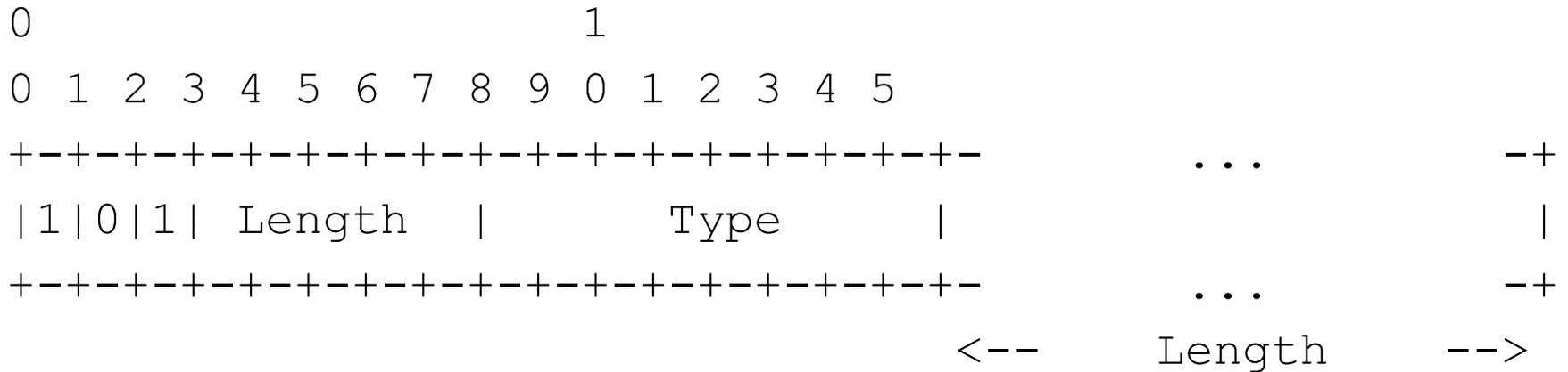
Elective format (above) is skippable thanks to standard length field whereas Critical format is not. Length is derived from Type/ Type Specific Extension
