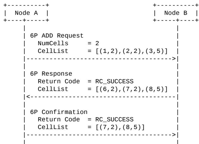
Figure 6: A 3-step 6P Transaction with cell suggestion.
