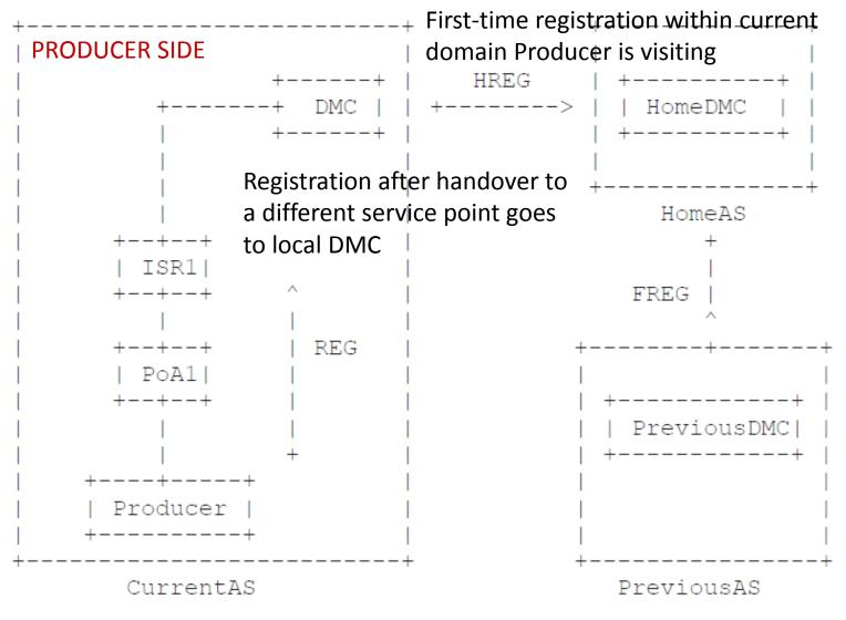
Inter-domain handover triggers timeout-based flushing of registration entries associated with Producer, and re-direct to new domain
