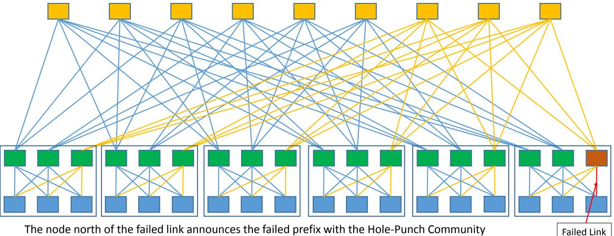
The node north of the failed link announces the failed prefix with the Hole-Punch Community on the yellow links in one spine plane. Receiving nodes will find the other routes with shorter netmask and prefer them instead.
