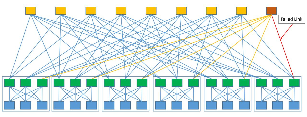
The node north of the failed link announces the failed prefix with the Hole-Punch Community. A single BGP route is sent on the yellow links in the north side of one spine plane.
