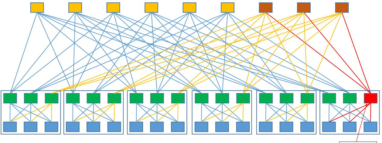
This is like multiple north side link failures. A single BGP route is sent on the yellow links in one spine plane.
