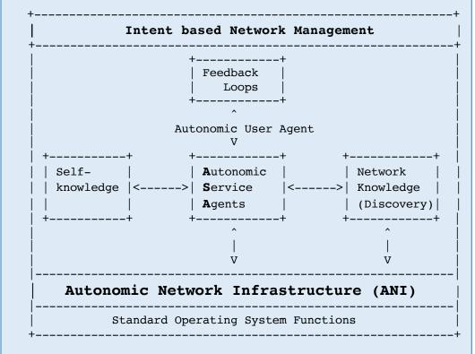
Figure 1: Reference Model for an Autonomic Node from RFC7575 slightly enhanced
