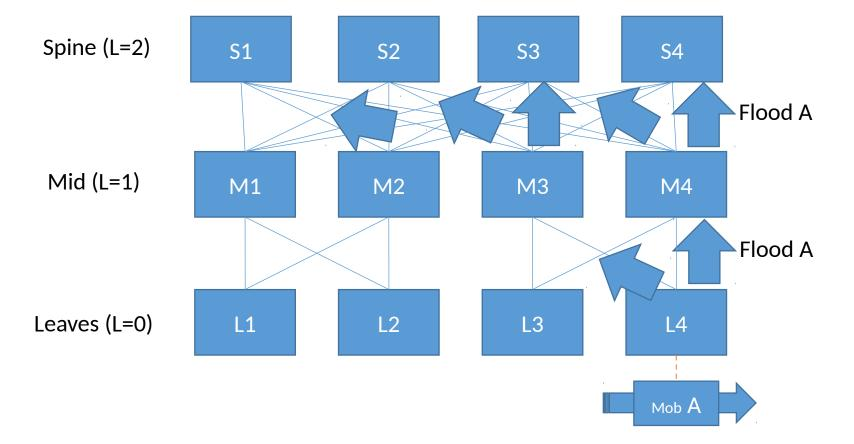
An alternate is to hybrid RIFT with a classical mobility approach based on dynamic tunnels to the attachment leaf. In that approach "mobile" N-TIEs are flooded to the superspine, no need to learn from them in intermediate levels As a result, <u>any superspine node can tunnel back</u> to the attachement leaf
