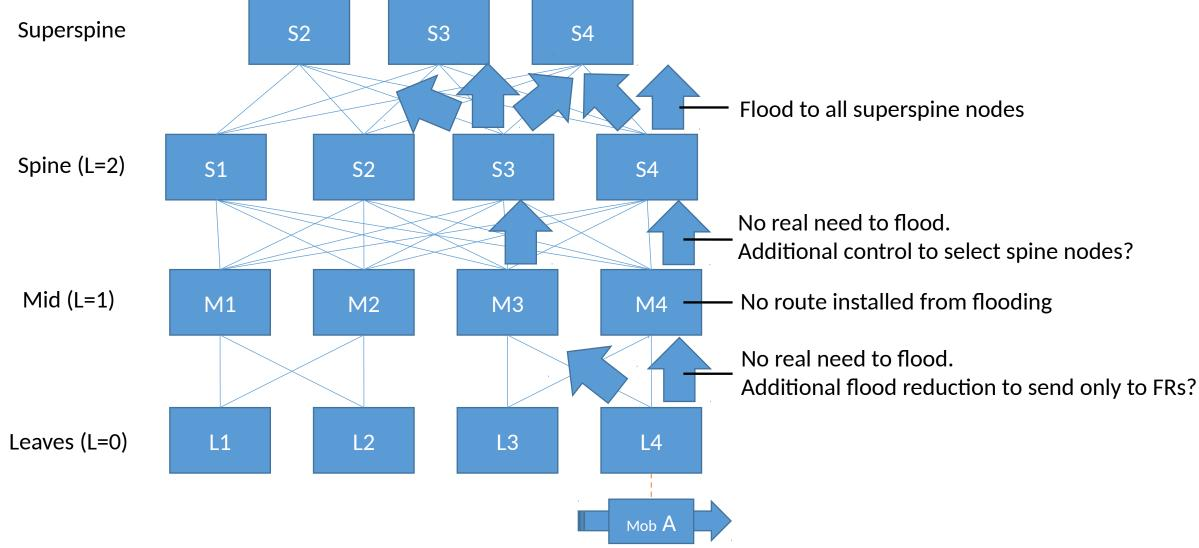
Since there is no knowledge of A south of it, packets eventually reach the superspine <u>on any superspine node</u> Any given superspine node can tunnel back; e.g., using Segment Routing (SR); all tunnels have a same cost/latency **pros:** fast, no stale route to clean up in the fabric; **cons:** longer path all the way through the fabric
