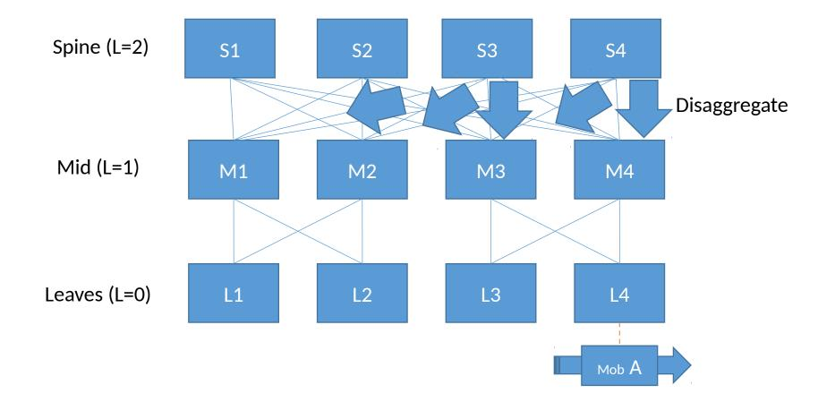
Since there is no knowledge of A but at the spine, packets to A get routed the spine along the more specific disaggregated route and then tunneled down by the spine to the attachment leaf
