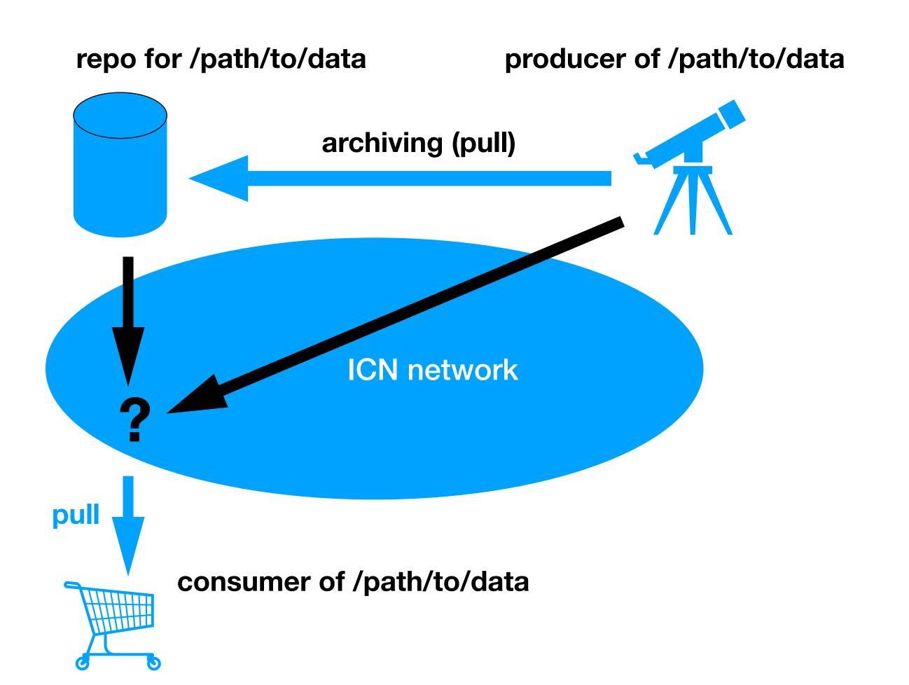
Config: streaming data is archived during recording, permits time shifting apps, also direct streaming.
