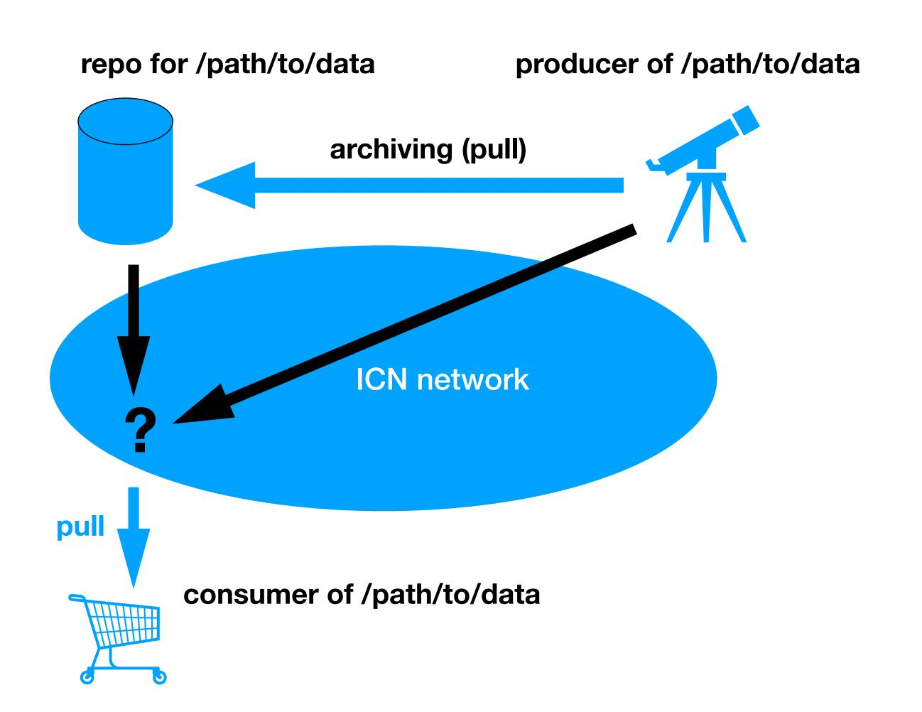
Config: streaming data is archived during recording, permits time shifting apps, also direct streaming.
