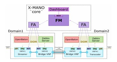
The aim is to show that the X-MANO is able to deploy network services with a negligible overhead and without imposing limitations on the underlying domains.
