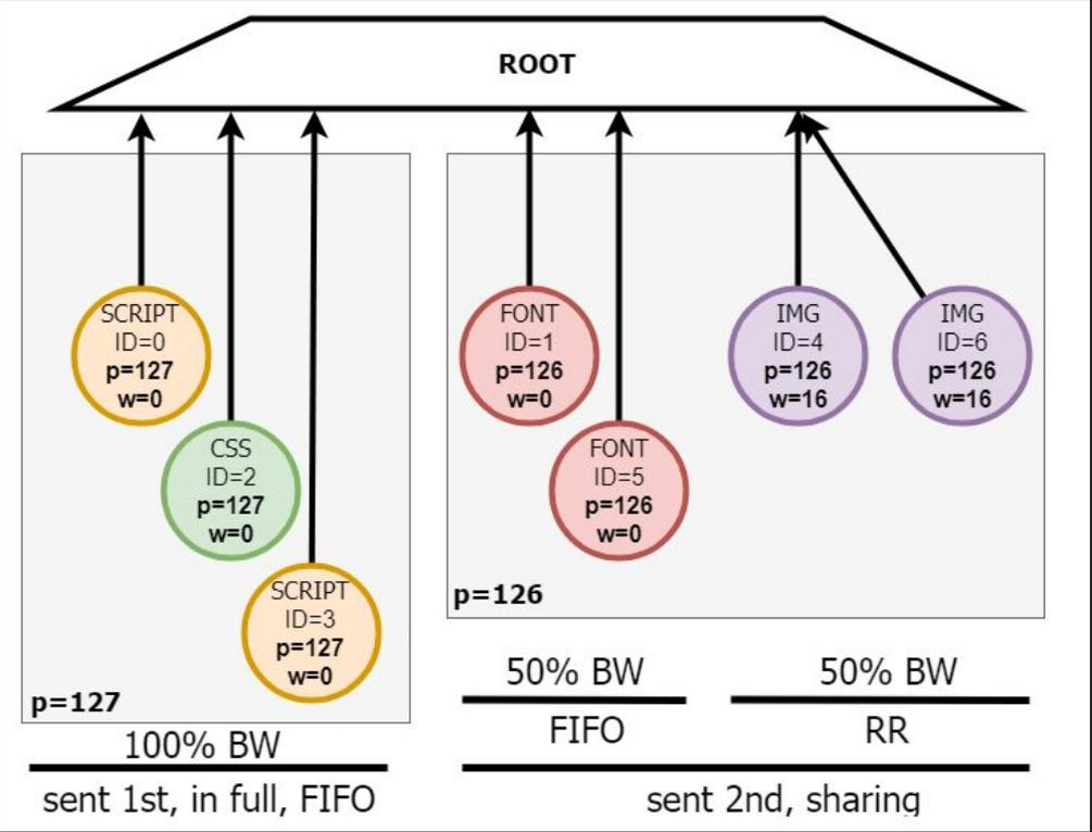
Allows FIFO and RR with hard ordering, without needing a single placeholder
