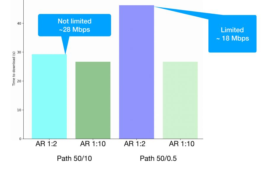
Measured with quickly for 100 MB transfer with AR1:2 and AR1:10 (flow credit was tuned) Return path: unconstrained (10 Mbps) and capacity-limited (500kbps)
