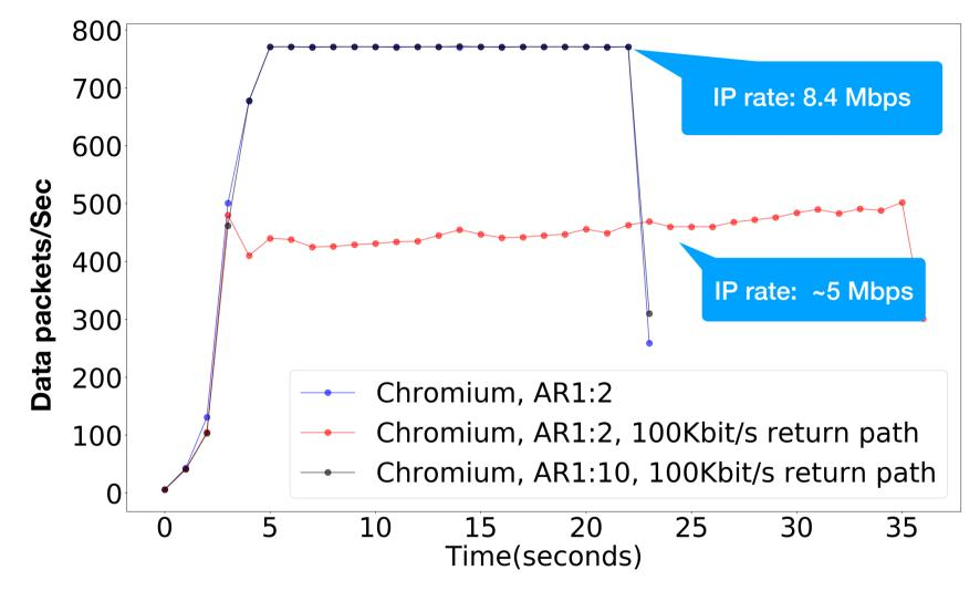
Measured data packets/sec using Chromium with AR1:2 and AR1:10 Return path: unconstrained (1.5 Mbps) and capacity-limited (100kbps) QUIC payload data size was 1350B; and IP QUIC packet 1378B.
