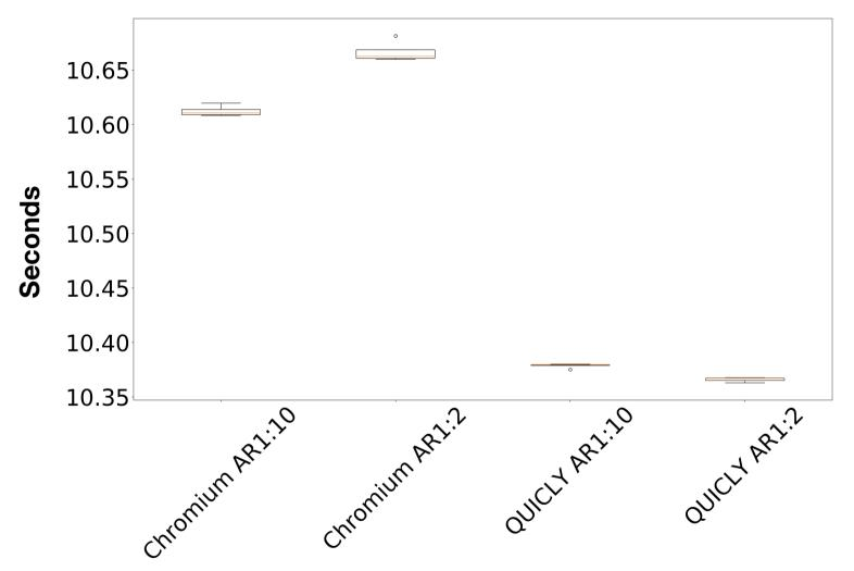
Time to download 10MB, emulated 20ms Path RTT, 8.5/1.5Mbps, n=6 transfers Note: Chromium uses AR 1:1 for the first 100 packets, Quickly does not, however this does not impact cwnd growth when RTT > delayed ACK value
