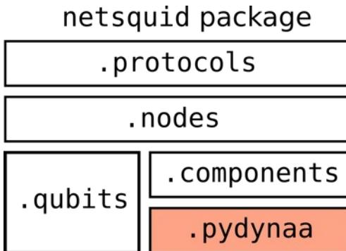
PyDynaa subpackage provides the **discrete event simulation engine**
