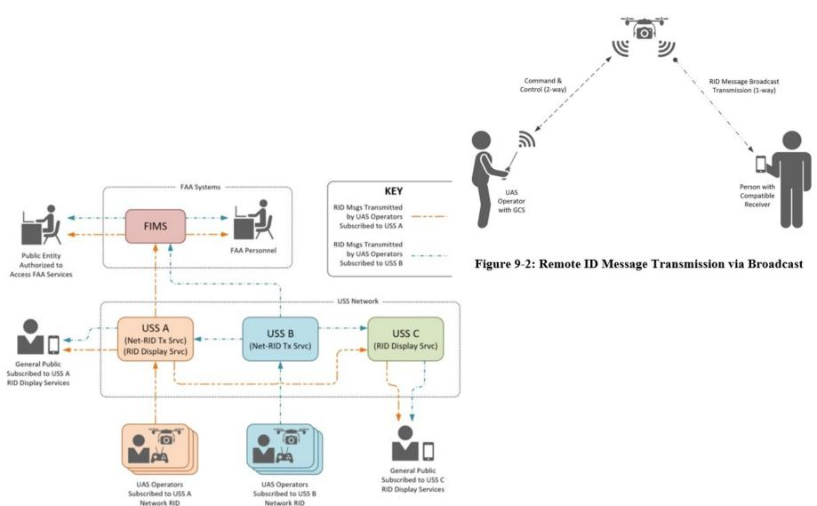
Figure 9-1: Remote ID Message Transmission via Network Publication Flow
