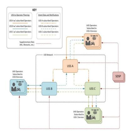
Figure 6-1: Notional High-Density Operations in UTM
