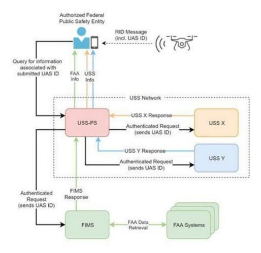
Figure 10-1: Direct Query to FAA and USS Network
