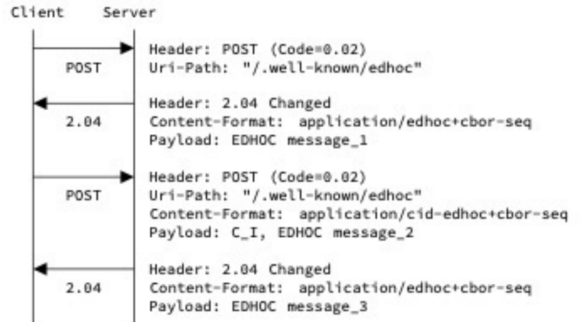
Figure 19: Example of the reverse message flow.
