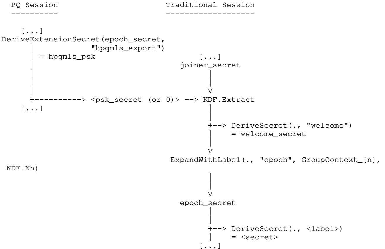
Fig 3: The hpqmls_psk of the PQ session is injected into the key schedule of the traditional session using the safe extensions API DeriveExtensionSecret .
